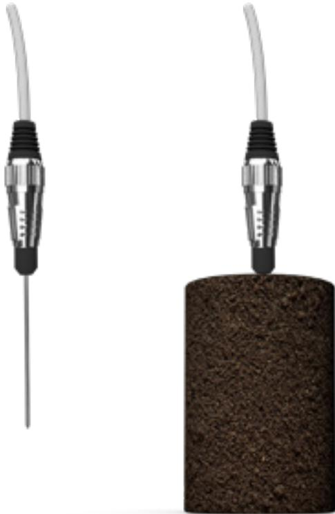
Each TLS-100 comes equipped with the standard 100 mm sensor for testing of soil, soft materials, viscous liquids and easy to drill materials. The needle sensor is fully inserted into an isothermal sample and a measurement is made with the push of a button. After 180 seconds, results are displayed for thermal conductivity and thermal resistivity. Saved results can also be exported to a computer, via Micro-SD card or USB connection.
